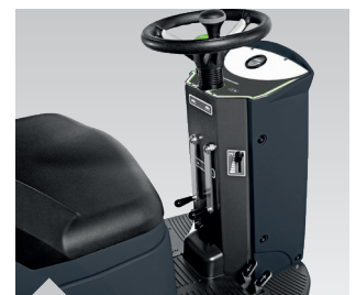
Mechanical operation of the brushes and suction bar via levers
