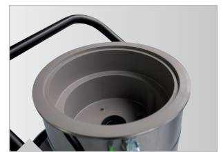
Protective insert with integrated float prevents liquid from entering the filters or suction motors during wet vacuuming
