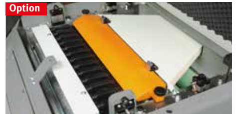
Fig. shows option "Pneumatic pressure setting of the upper feed rollers" for PS 630
