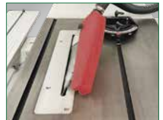
Saw blade tilt from 90° to -45° to the right
