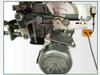
Solid saw unit guarantees vibration-free and precise work
