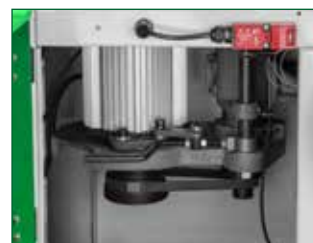
Quick and easy speed change by means of multi V-belt
