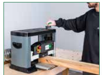
Height adjustment via hand crank and scale
