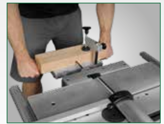
Slot mortising device For the simple production of grooves, mortises and Plug connections
