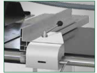
Large aluminium rip fence on round rod guide with fine adjustment
