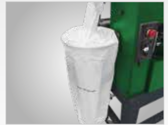
Integrated extraction system for dust-free working
