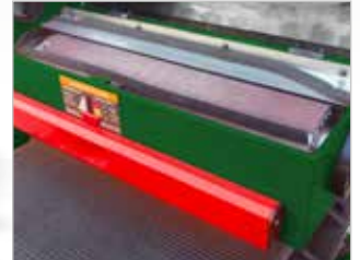
Solid steel roller and built-in safety switch on the feed side
