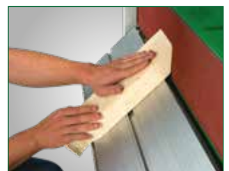
Mitre cuts up to 45° by swivelling the longitudinal table
