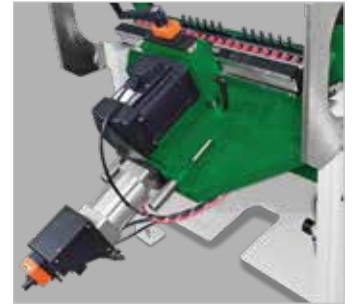
Drilling unit Pneumatically swivelling to 45 and 90 degrees
