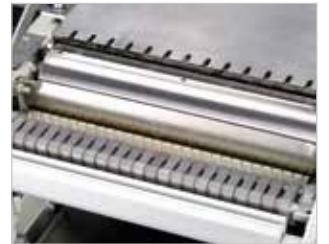
Automatic, even feed with kickback protection. The toothed feed roller ensures a constant wood feed.
