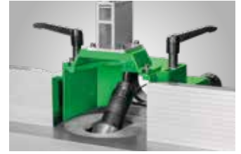
Milling spindle can be swivelled to the rear for optimum use of a feed attachment, maximum safety and a clean milling pattern
