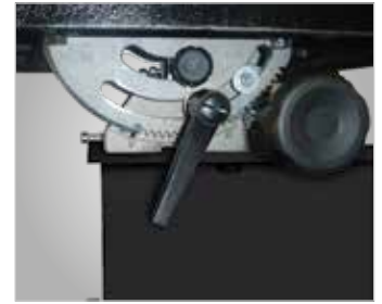
The saw table can be tilted from 0° to 45° on a rocker support
