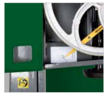
A viewing window integrated into the door allows you to check the saw band tension from the outside.
