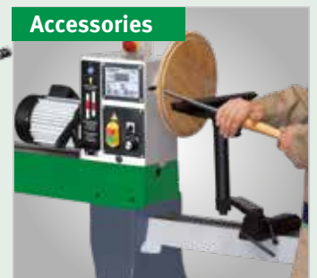
The headstock can be swivelled to turn workpieces in cross-grain operation that are larger than the bench's turning diameter. The bed extension in combination with the reversible tool rest enables maximum flexibility.
