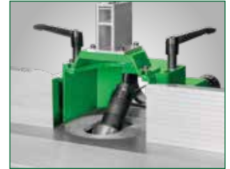
with swivelling milling spindle -5° to +30°
