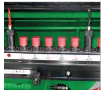
21 Drill spindles Six quick-change drill chucks for 10 mm shank included in delivery
