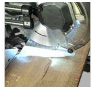
Extremely precise light projection of the cutting edge
