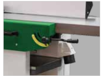
Surface planing Simple adjustment of chip removal up to 3 mm via operating lever.
