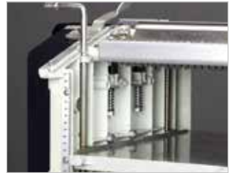
The spring-mounted feed rollers prevent indentations on the wood. The thickening table is guided on four pillars.
