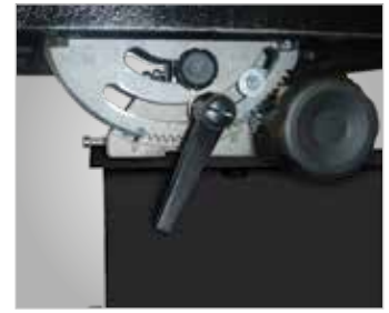
The saw table can be tilted from 0° to 45° on a rocker support
