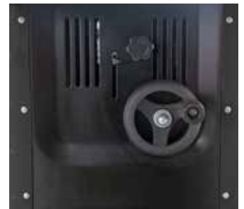
Spindle height adjustable from 0 to 40 mm
