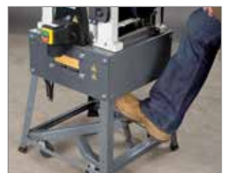
The standard chassis with two swivel rollers enables easy transport. To move the machine, simply step on the chassis bracket, which brings the rollers down. The undercarriage returns to its original position via a spring bar.
