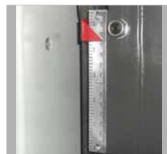
Set height of the worktable can also be read off the scale
