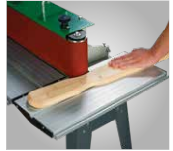
Mitre cuts up to 45° by swivelling the longitudinal table
