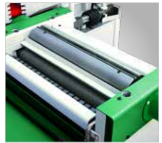
Precision-mounted blade planing shaft with reversible blades
