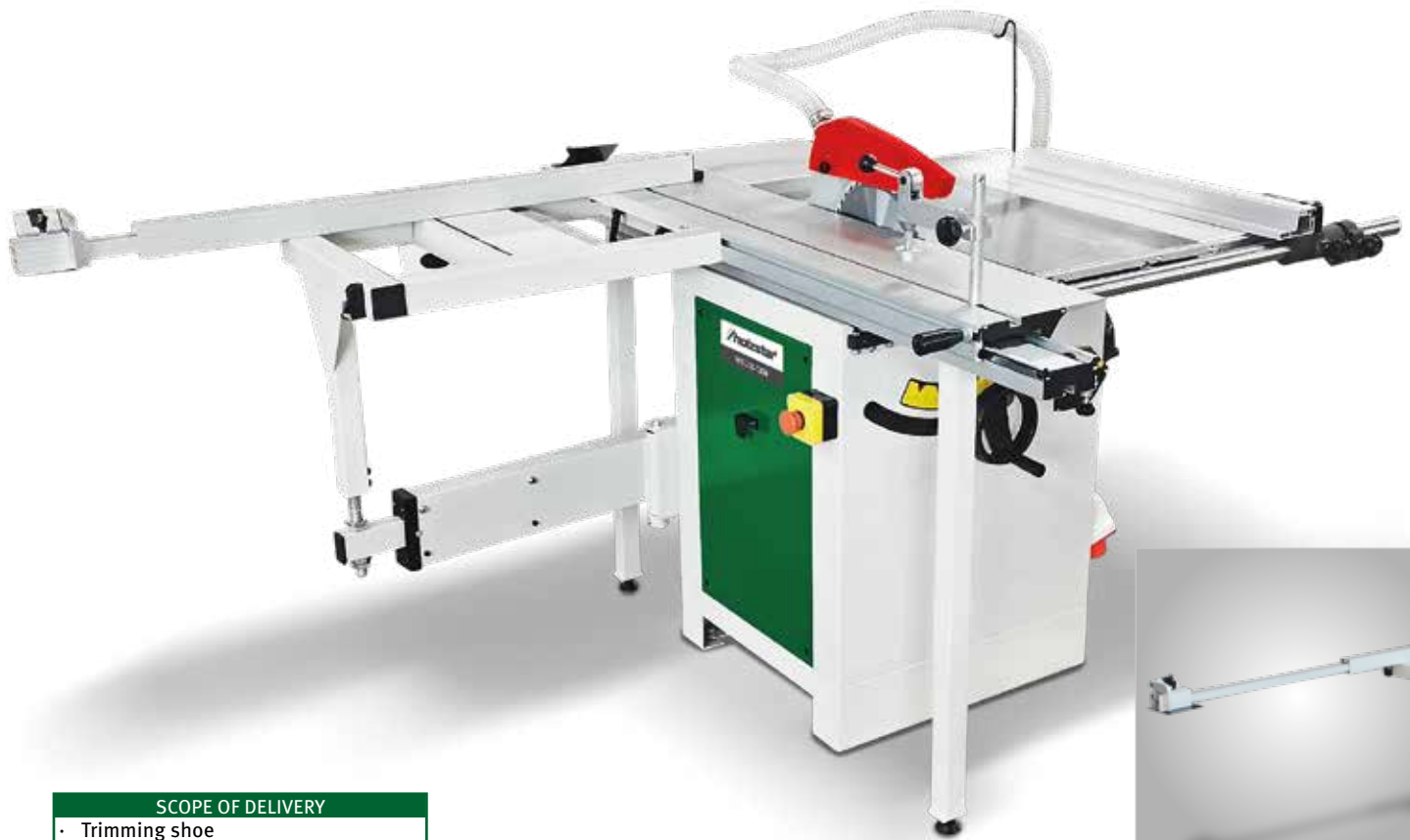
Telescopic fence with a length of 1100 to 1900 mm
