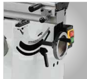
Handwheel for height adjustment of the saw blade
