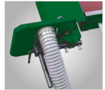
Height-adjustable supplementary table with suction, for sanding inner radii
