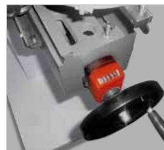
Convenient, precise table height adjustment via a handwheel with numerical display
