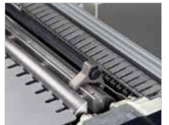
The planing knives are adjusted using the planing knife adjustment gauge supplied.
