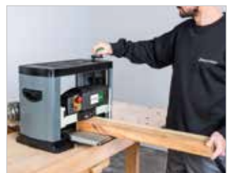
Height adjustment via hand crank and scale
