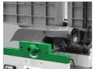
Fixed extraction bonnet The fixed extraction hood means there is no need to reconnect the extraction hose during conversion. Time-saving
