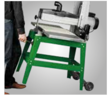
Movement device for easy relocation of the machine
