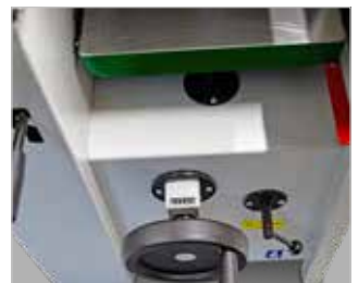
Thicknessing table Guide on centre pillar and additional guide Height adjustment via handwheel Height display by mechanical counter with 0.1 mm accuracy
