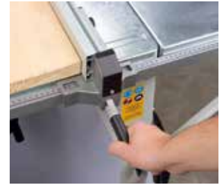
The rip fence with eccentric quick clamping can be adjusted precisely and easily using a scale.
