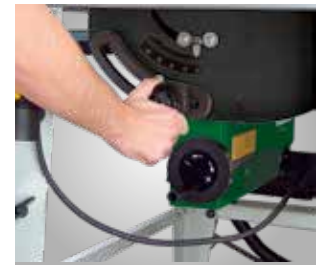
With precise and smooth height and tilt adjustment of the saw unit using easy-to-operate handwheels.
