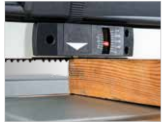
Mechanical display of chip removal
