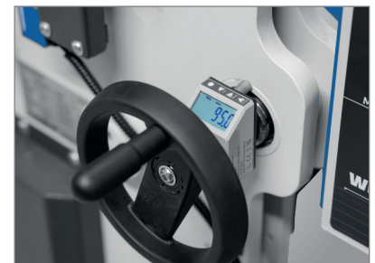
Adjustment of the rear stop via handwheel with counter
