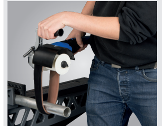
▶ Satin finishing of round steel with Velcro fleece, even with already installed stainless steel railings, for example
