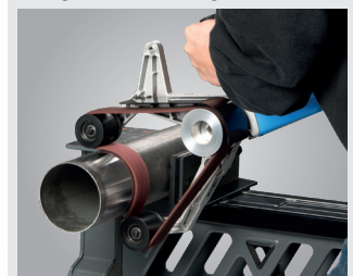
▶ Only two work steps necessary for 360° peripheral sanding
