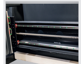
▶ The X-axis, driven by ball screws, runs on double linear guides
