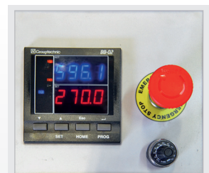
▶ Simple operation, with digital display for current bending values and for setting the parameters
