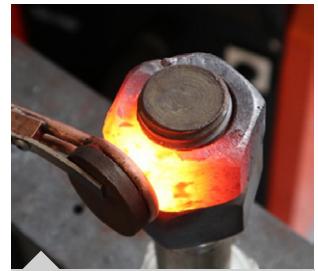
Preheating before welding
