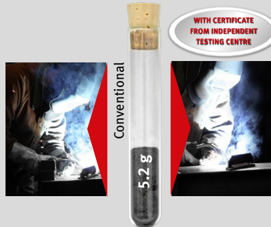
Welding fumes produced when welding 1kg of SG wire
