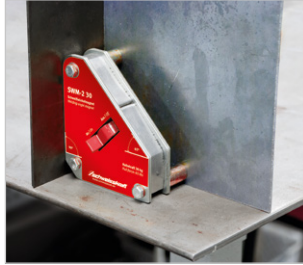
For holding metal workpieces at a 45° or 90° angle
