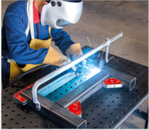
For holding metal workpieces at a 45° or 90° angle
