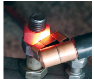
› Heating a nut with the focus coil at an angle
