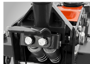
› Quick-Lift function with double piston
