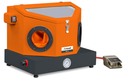
SSK 1.5 ▶ Regulation of the working pressure via pressure regulator with pressure gauge ▶ Air flow is controlled via foot pedal ▶ 12-volt fluorescent tube with 230-volt power supply unit and external switch ▶ Integrated extraction system with replaceable air filter
