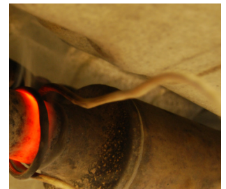
› For loosening parts that are difficult to access using special winding wire
