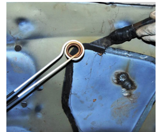
› For easy removal of smaller panelling
